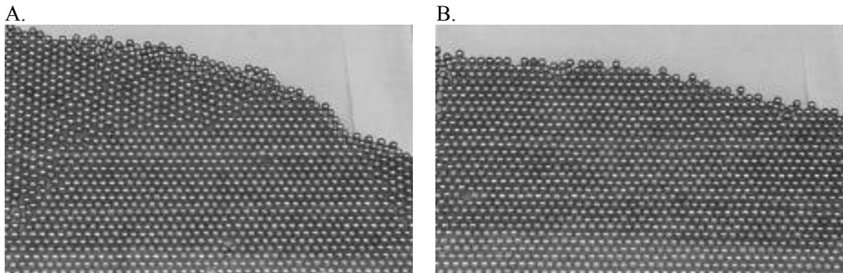
Figure 1. BB board with defects (A), and without defects (B).
