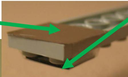
refrigerator magnet probe taped to cantilever (magnetic pole stripes parallel to cantilever and facing downward)
