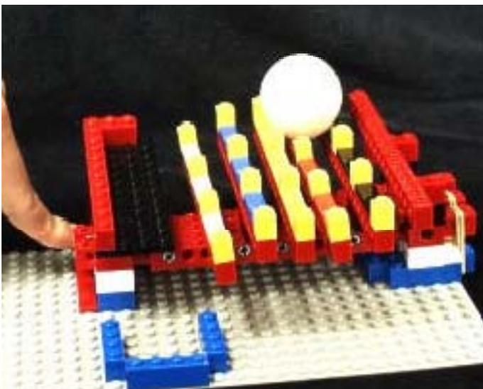
A table tennis ball (representing an electron) can be placed anywhere on the platform. The different smooth sites represent electrodes in a CCD array. Slowly press and slowly release the levers in sequence (this represents changing the voltages on the electrodes) to move the ball to the ramp. The ramp represents the readout register of the CCD.
