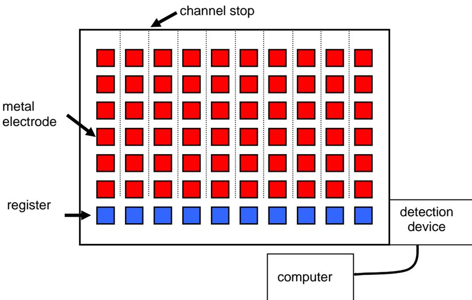
Figure 2.4 – Electrode array of a CCD.
