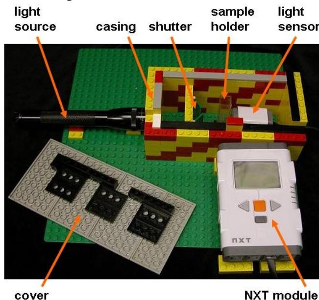
Figure 2.9 - A LEGO<sup>®</sup> photometer. See Section 2.3 Appendix for building instructions.
