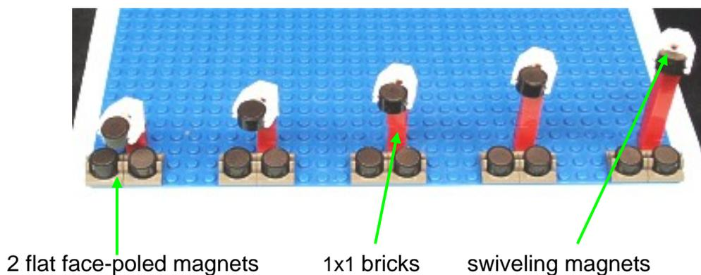
Figure 2.13 – Setup for the LEGO® pulsed NMR experiment.
