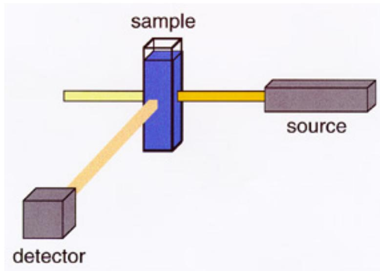
Figure 2.12 - The 90<sup>o</sup> geometry for light scattering measurements
