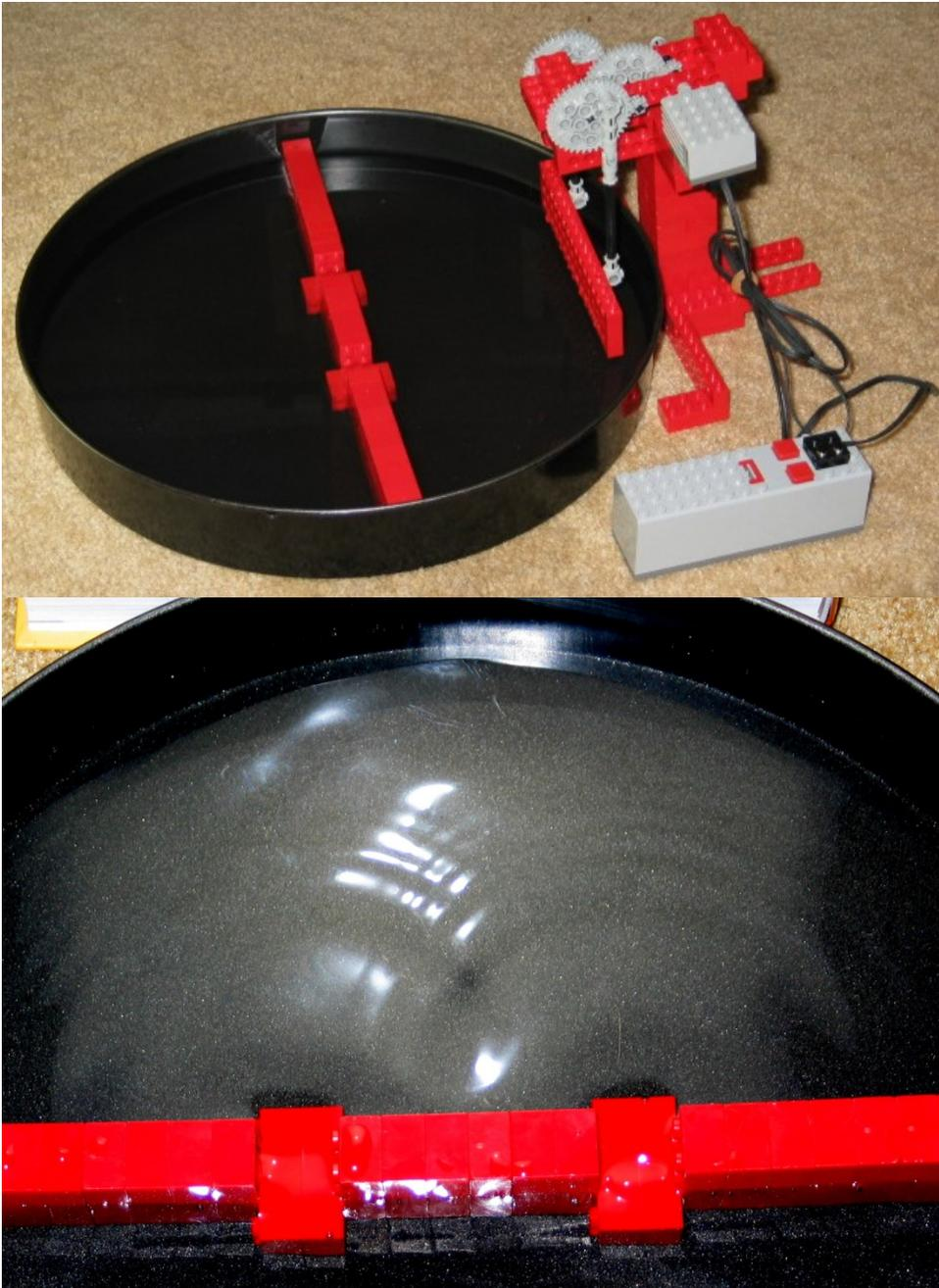
Figure 2.20 – (top) A wave tank made using LEGO® bricks and a flat pan filled with water. A long, straight wave can be produced by oscillating a flat wall of LEGO® bricks. The wall can be oscillated up and down by using a LEGO® machine or by hand. (bottom) Interference between sets of circular waves scattered from two gaps in the 2x4 LEGO® brick barrier. The water level is lower than the bricks oriented vertically but higher than the bricks in the gaps that are oriented horizontally.
