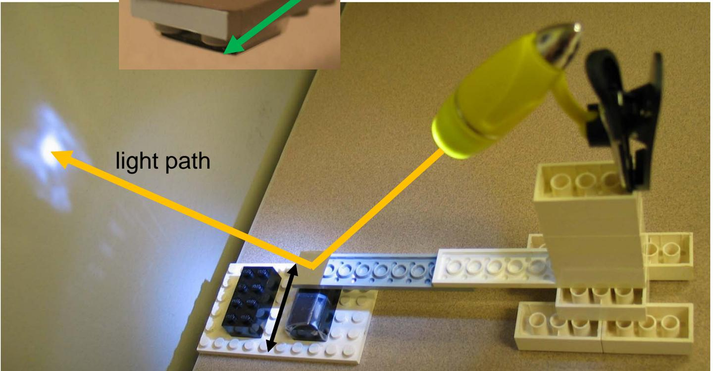
Substrate is a refrigerator magnet taped to a regular brick on a flat brick. Substrate motion is perpendicular to magnetic pole stripes in the substrate and the cantilever as well as the light path.
