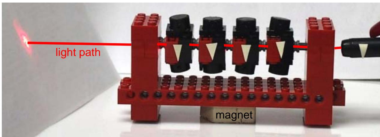
When a very strong magnet is placed under the platform, the magnetic units will all align in the same direction, allowing light to pass through the holes in the LEGO beams.
