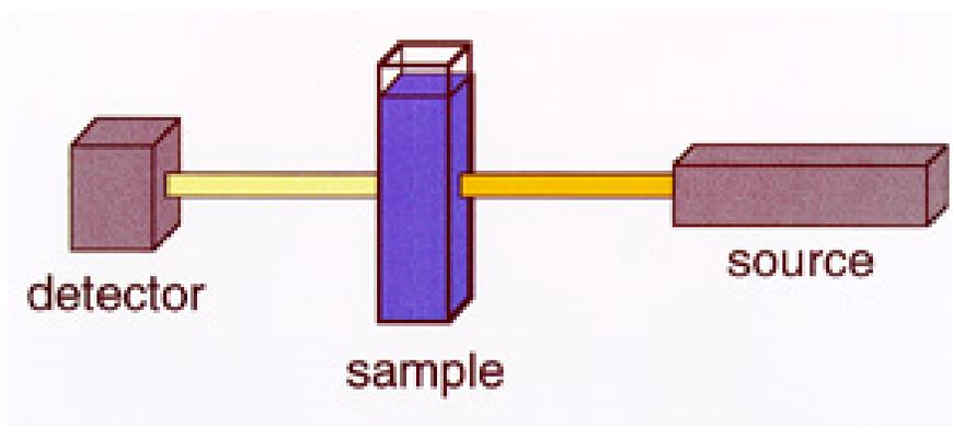
Figure 2.8 – General schematic of a photometer.
