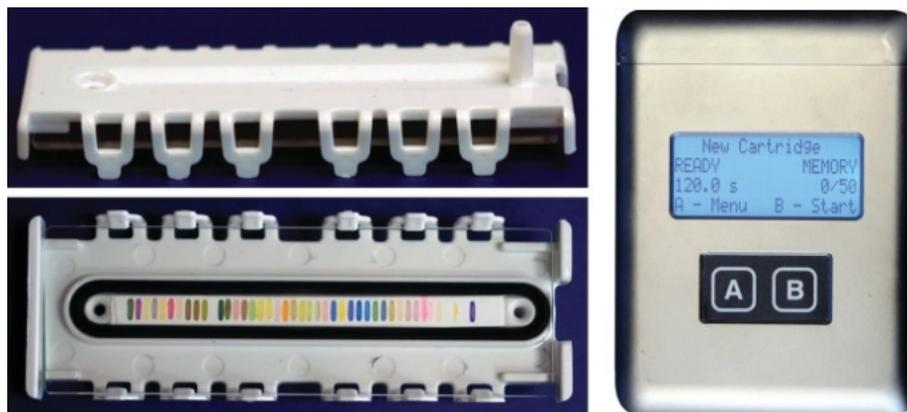
This optoelectronic “nose” (side and front views, left) and handheld reader-analyzer (right) detects TATP and many other compounds on the basis of the response of an array of colorimetric sensors embedded in a disposable cartridge. Credit: Chem. Sci.
