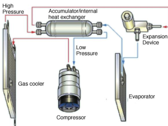
**THE COMPETITION** Auto air conditioners could soon depend on CO<sub>2</sub>, as does this newly designed system from component supplier Visteon.
