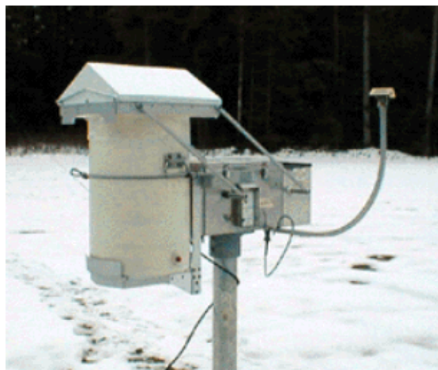
Figure 5-1: An Environment Canada Acid Precipitation Collector
