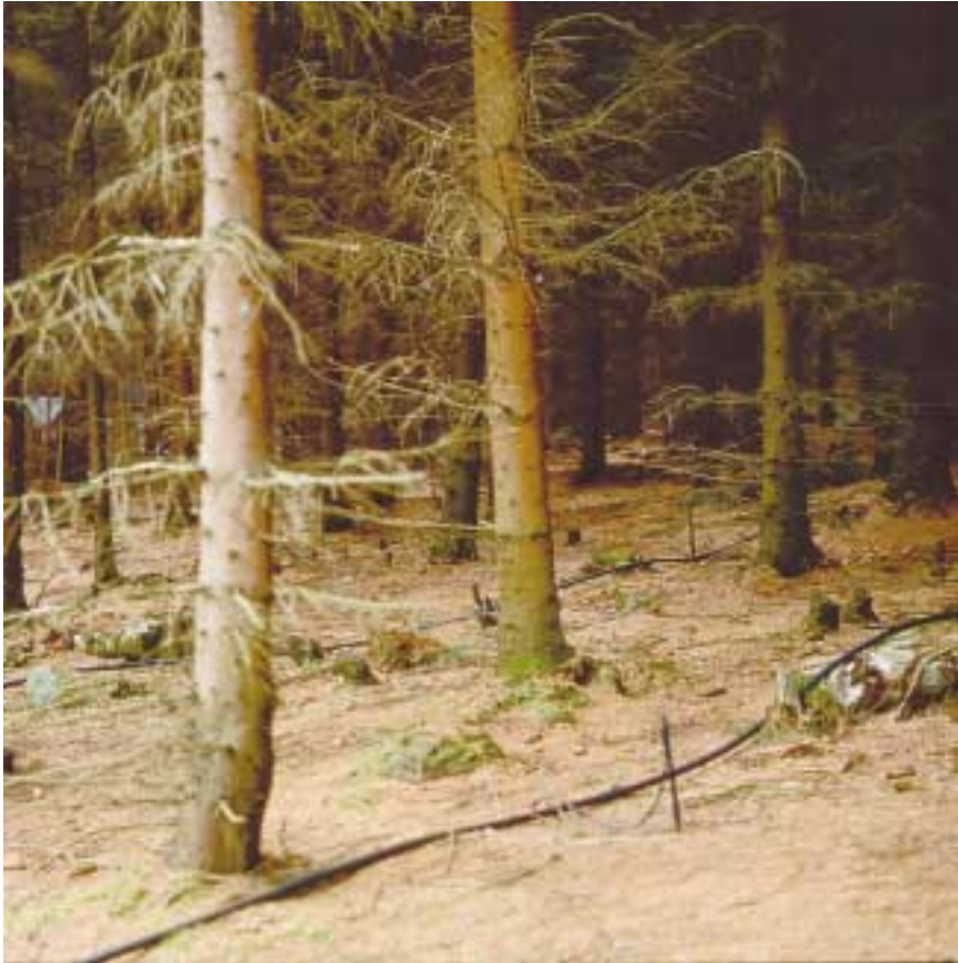
The Skogaby experiment in south-west Sweden has been set up in a young Norway spruce forest with sparse undergrowth (mostly forest bryophytes). This photograph, taken in May 1997, shows the tubing and sprinklers used to apply a nutrient solution in one of the seven experimental treatments. Photo: Tryggve Persson.
